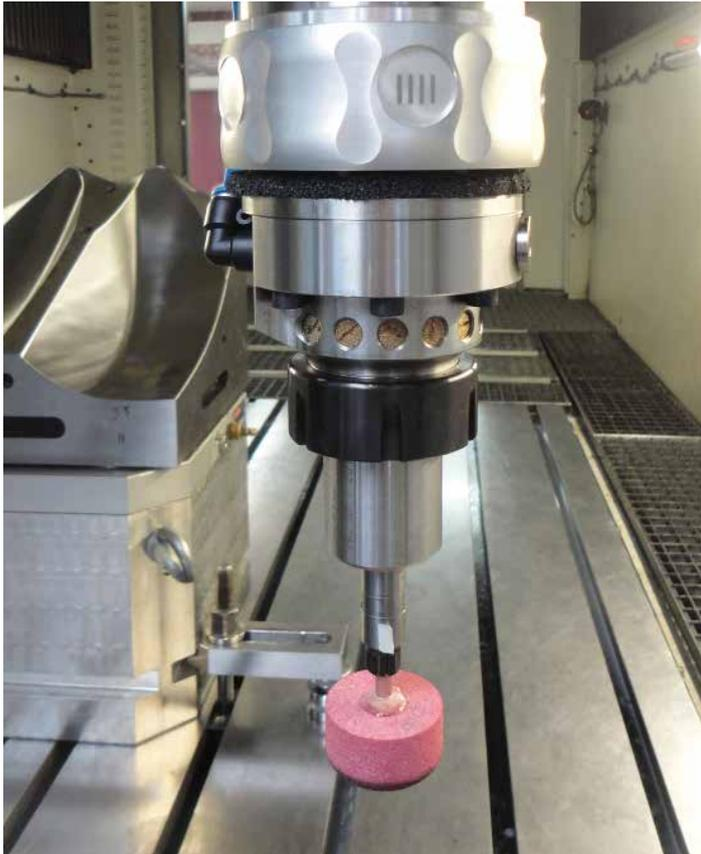
**T**he experts for pneumatic tools and spindles from Biax, a trademark of the Swabian family-owned company Schmid & Wezel from Maulbronn, have brought to the market the modular pneumatic spindle system „RSC“ with a deflection unit that could fundamentally change the polishing and refinishing of surfaces.
